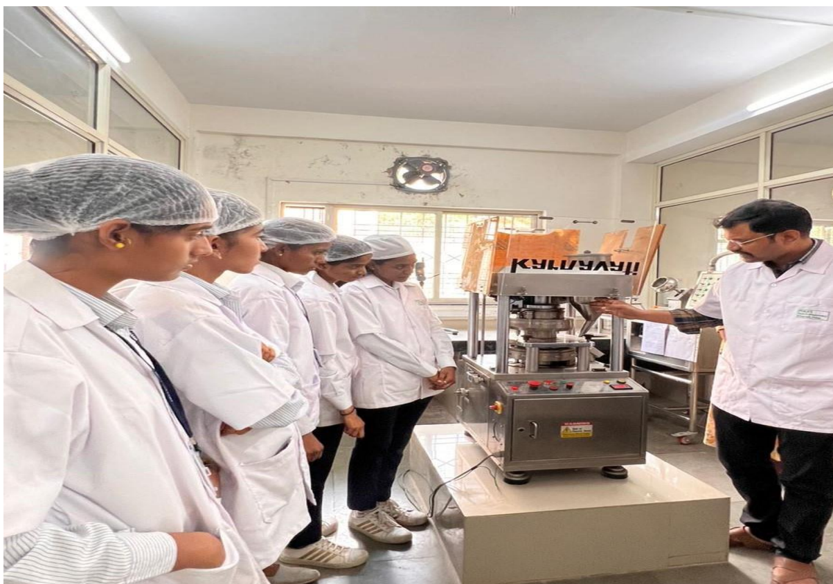
Dr. Sujit Kakade explaining the students about working of rotary tablet punching machine
